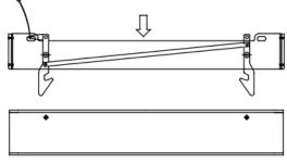
• Bring down the Lifting Device until it engages the log (the Lifting Device hooks will open when they contact the log's lifting hinges and will close by its own weight after moving down passed them).
